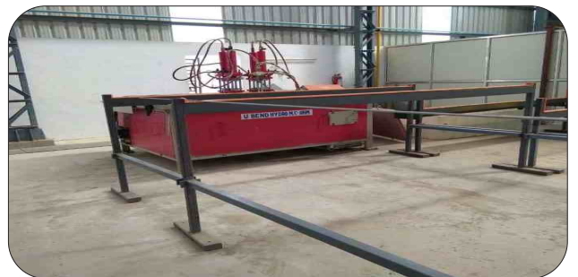
U-BEND HYDRO MECHINE
