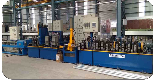
TUBE MILL WITH ONLINE BRIGHT ANNEALING AND EDDY CURRENT
