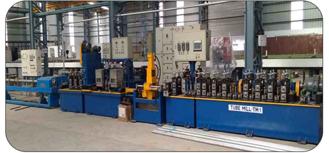
TUBE MILL WITH ONLINE BRIGHT ANNEALING AND EDDY CURRENT
